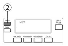
When you select a new programme, the maximum temperature is shown on the electronic display.
